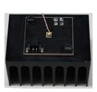
Picture 5. Fins facing down (Nichia uses this orientation) (This orientation obstructs the air flow)
