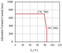
Figure 1.  $T_S$  vs Allowable Forward Current
